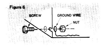
• If necessary, drill 3/16" diameter hole in cabinet for ground wire (see Figure 7). Place remaining length of wire under front lip of base behind plastic front panel.
